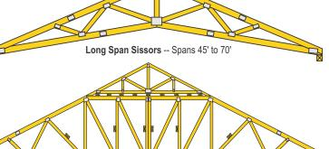
Three Piece Long Span (Field Connected) -- Spans 60' to 80'
